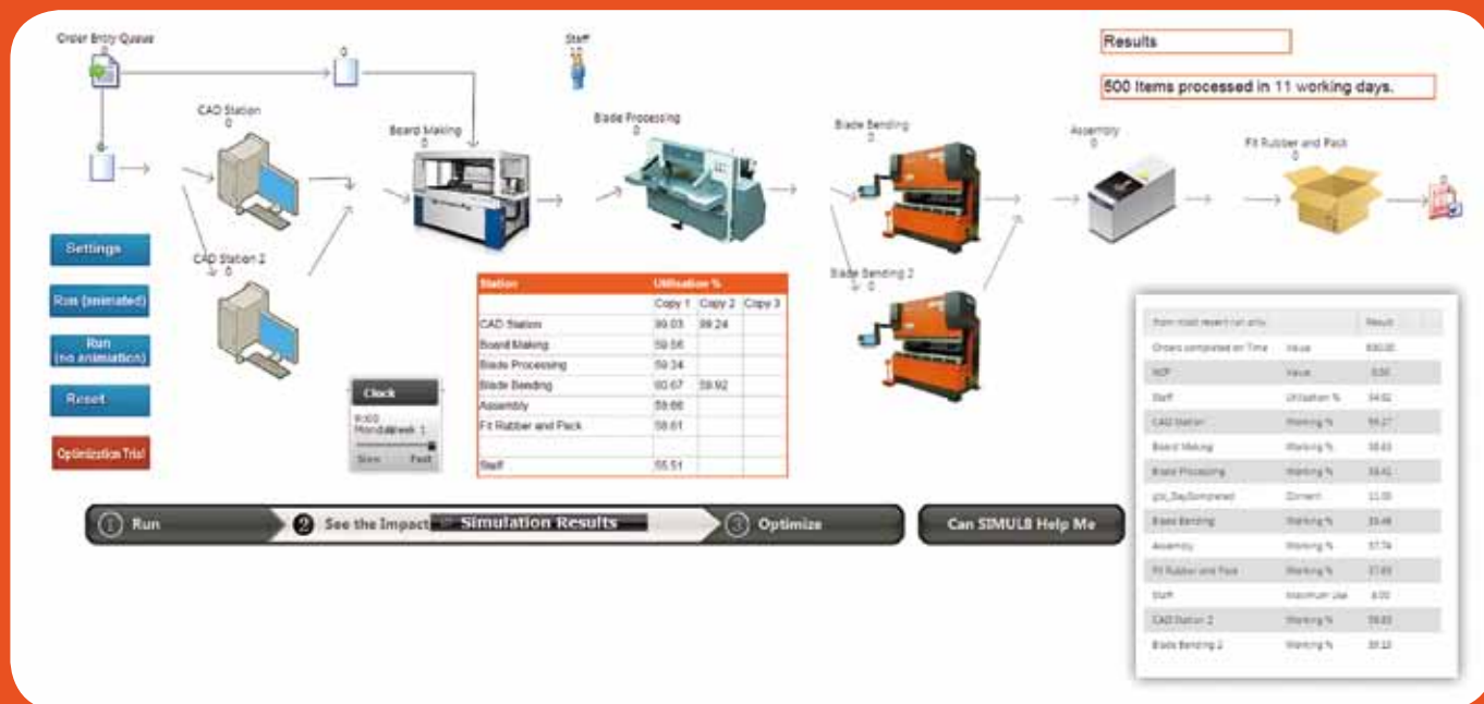
Figure 1: Addition of extra machines at the blade bending process. Experiment to reduce bottlenecks regarding investment planning.
